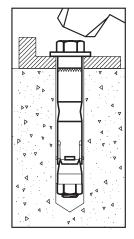
3. Drive anchor through the fixture into the hole. Be sure the anchor is driven to the minimum required embedment depth,  $h_{nom}$ .
