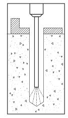
2. Remove dust and debris from the hole using a hand pump, compressed air or a vacuum.
