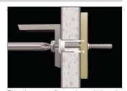
Place item over flange. Insert bolt and tighten until snug against item, then stop. Use machine screw or bolt to match thread in metal channel.
